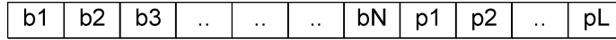
Fig. 7. Memory word organization for the proposed error detection code for N/L integer.
