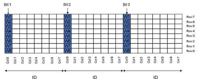
Fig. 1. Example of Interleaving in a memory.
