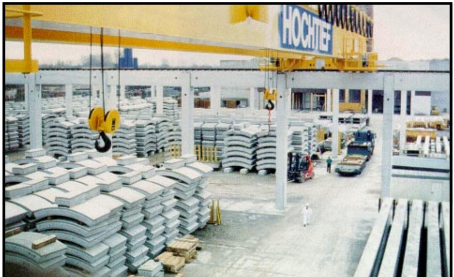
Photo 1 —When transporting concrete modules for bridges and tunnels by a crane, sway of the load must be controlled. A fuzzy-logic controller uses the experience of a human crane operator. This crane has two heads, each capable of transporting 64 tons, and it employs an antisway controller based on fuzzy logic.
